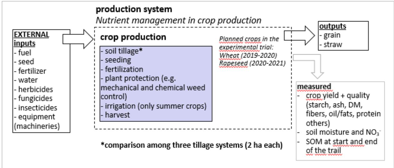
**Figure 8:** System under study – Conservation tillage to increase water- and nutrient use efficiency and its effect on soil quality characteristics – conducted in IT.
