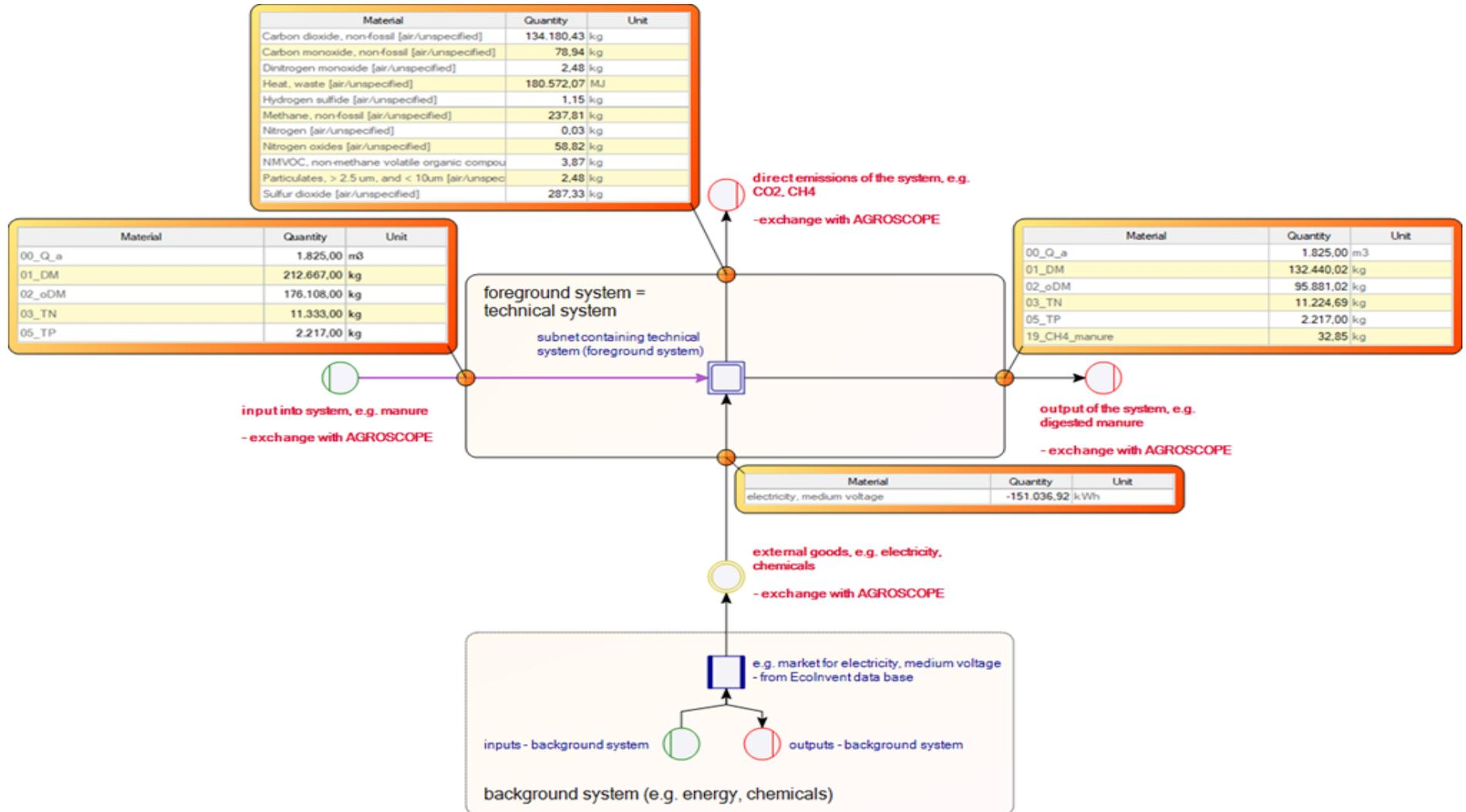
Figure 2: Exemplary flow-scheme of Umberto LCA + main-net with illustrated input and output flows.
