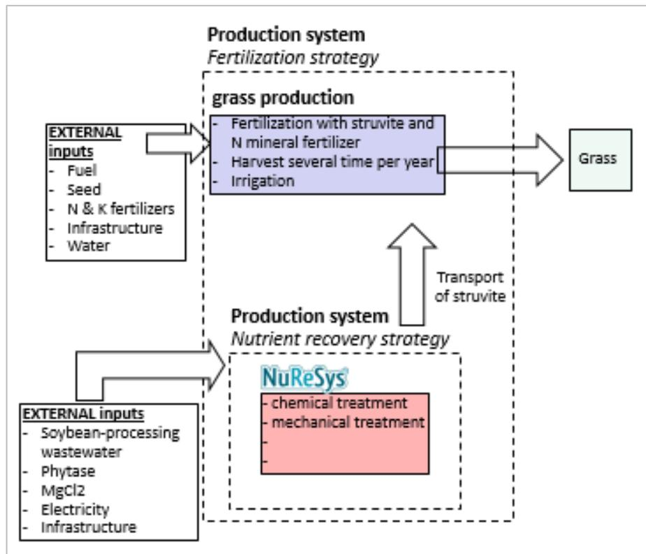
Figure 18: System under study – production of novel P fertilizers from Soybean wastewater in the NuReSys plant and field test of novel fertilizers in intensive grasslands – conducted in NL.
