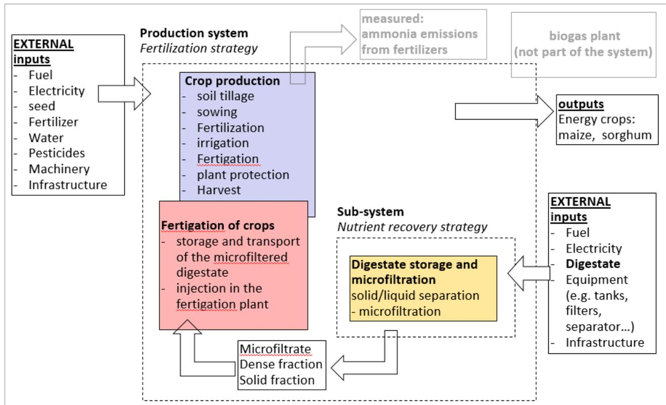
Figure 12: System under study – microfiltered digestate applied to energy crops by fertigation to reduce mineral N fertilization – conducted in IT.
