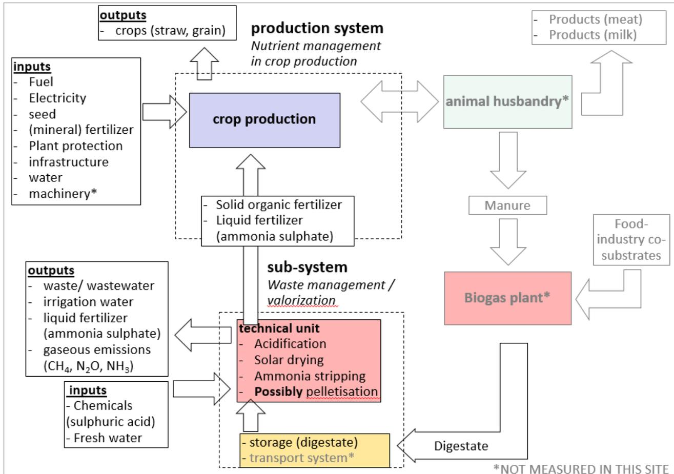
Figure 10: System under study – Fertilizer production from digestate by solar drying and testing of produced fertilizers in two different crop rotations – conducted in ES.
