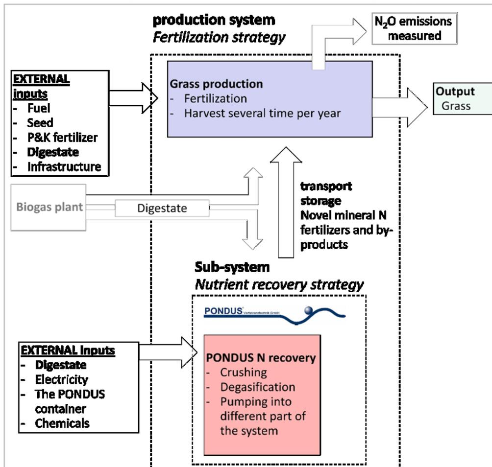
Figure 16: System under study – production of novel N fertilizers from different substrates in the PONDUS plant and test of different substrates in field experiments – conducted in NL.
