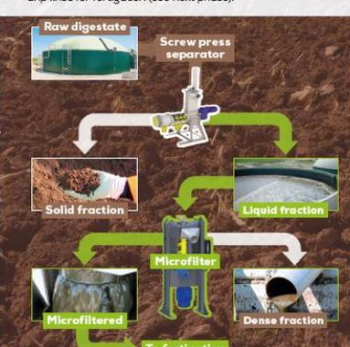
Flow rate microfilter: 4-5 m<sup>3</sup> of microfiltered digestate per hour.
