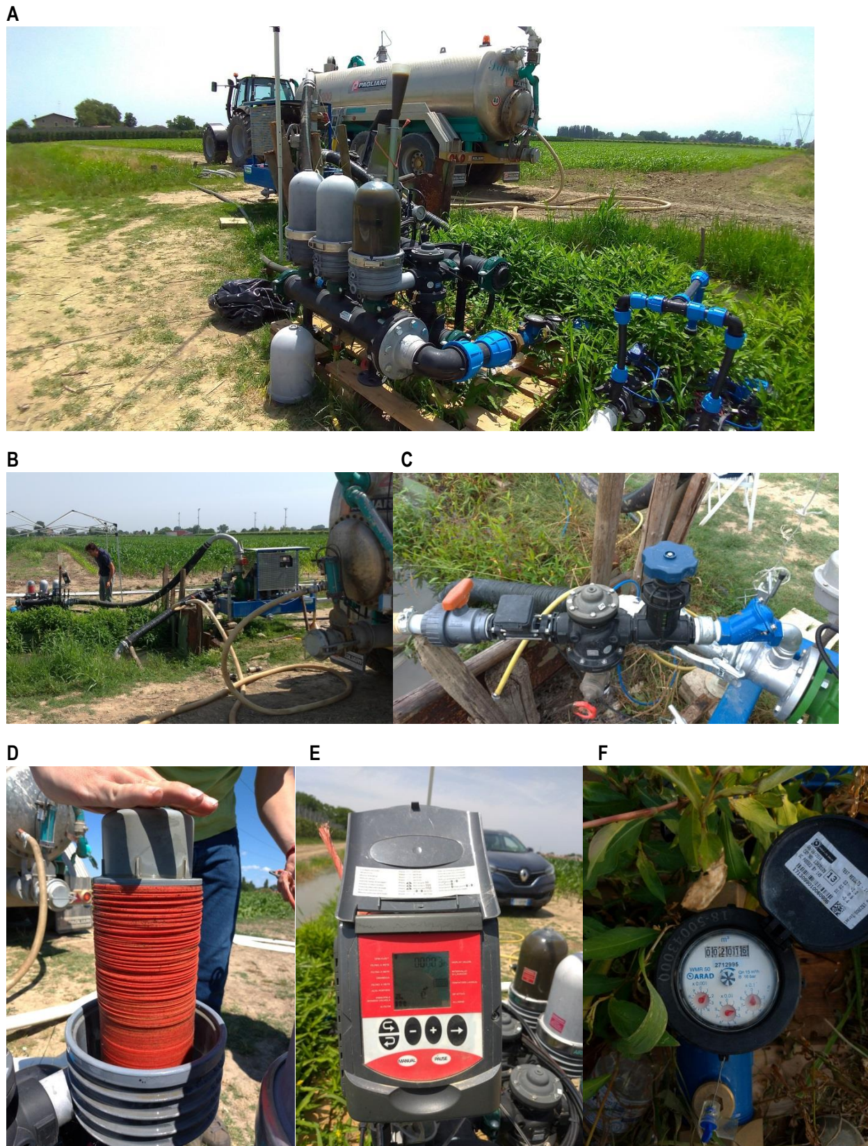
Figure 5: The fertigation plant with the microfiltered digestate tank and the disk filtration (A), the motor pump and the injection system for microfiltered digestate (B, C), the disks inside the filters (D), the filtration control unit (E) and a water meter (F).
