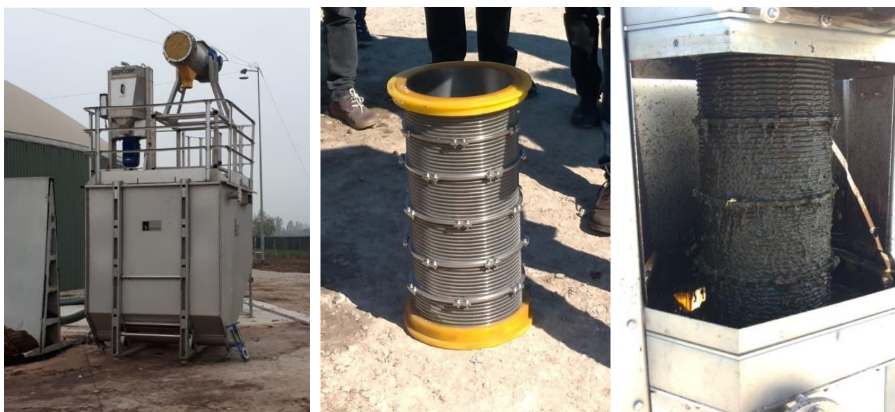
Figure 1: The solid/liquid separator + microfilter installation (left), the screen of the microfilter (centre) and the microfiltration of digestate (right)
